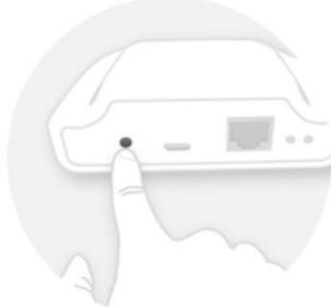
In order to find your SmartBox, press the button located at the front side of the device. Please make sure that it is correctly connected to your WiFi network.
